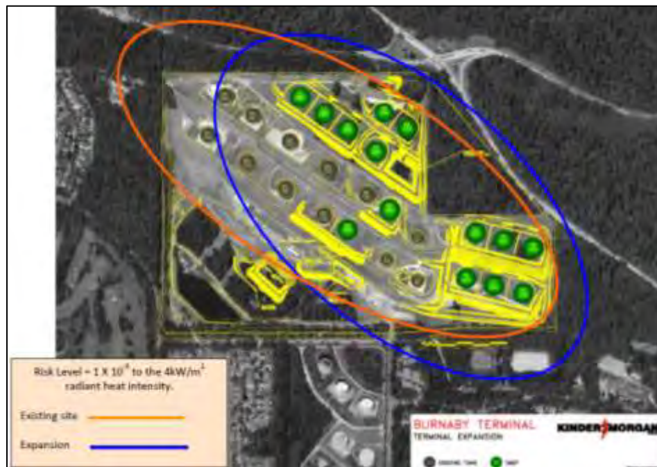
Figure 10.2: Summary of Risk Distances for Radiant Energy from a Dike Fire (for the existing site and expanded site)
